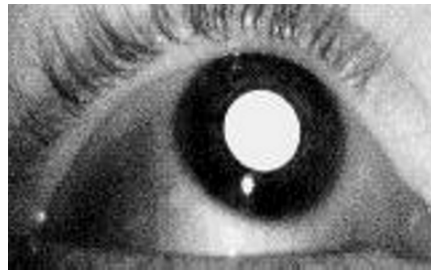
(d) Example of “bright pupil” (and corneal reflection) illuminated by infra-red light. Courtesy of LC Technologies, Fairfax, VA < http://www.eyegaze.com >. Reproduced with permission.
