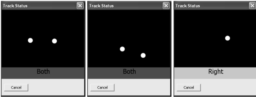
Fig. 11.1. Tobii eye tracking status window: sitting level; too far back with head tilted; left eye closed.
