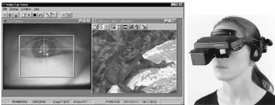
Fig. 5.6. Example of head-mounted video-based eye tracker. Courtesy of IOTA AB, EyeTrace Systems, Sundsvall Business & Tech. Center, Sundsvall, Sweden < http://www.iota.se >. Reproduced with permission.
