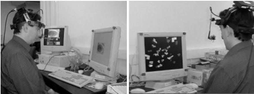
(b) An eye-tracker is used to determine the viewer's point of fixation.
