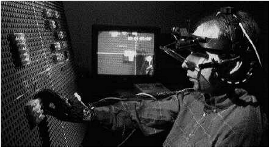
Fig. 17.8. Eye tracking in a natural pick-and-place task. Courtesy of Jeff Pelz, Visual Perception Laboratory, Carlson Center for Imaging Science, Rochester Institute of Technology < http://www.cis.rit.edu/people/faculty/pelz/-research/ASL_tracker.html >. Reproduced with permission.
