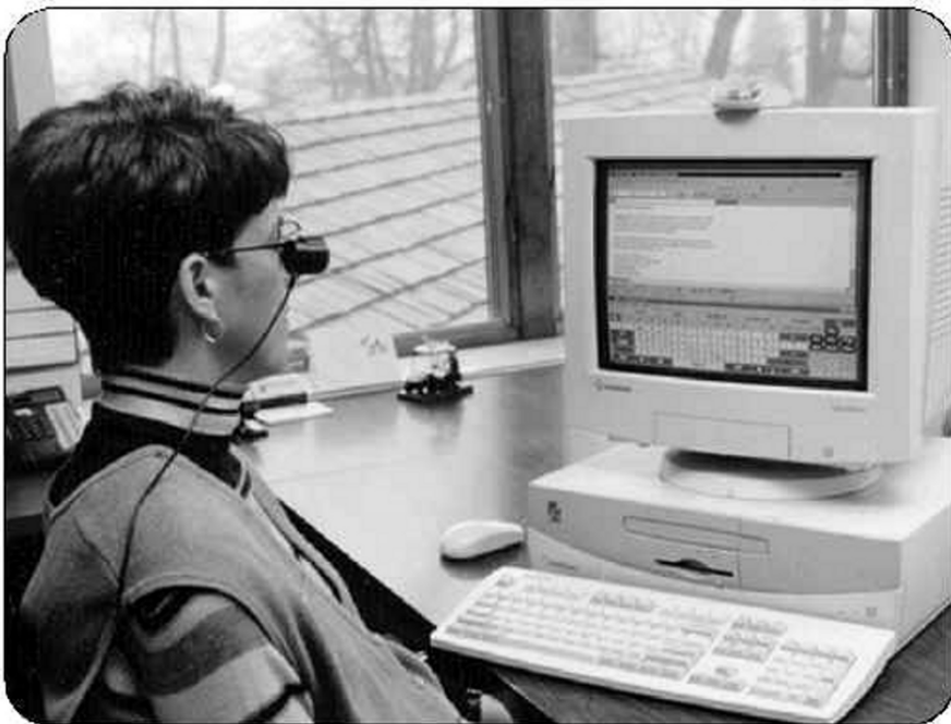
Fig. 20.2. Example of eye typing interface. Courtesy of Prentke Romich Company, Wooster, OH < http://www.prentrom.com/access/hm2000.html >. Reproduced with permission.
