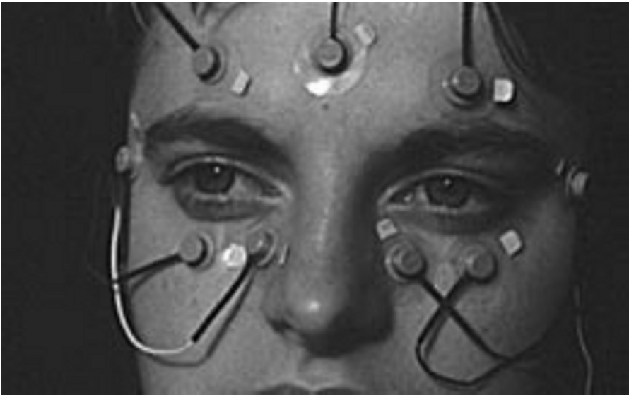
Fig. 5.1. Example of electro-oculography (EOG) eye movement measurement. Courtesy of MetroVision, P erenchies, France < http://www.metrovision.fr >. Reproduced with permission.
